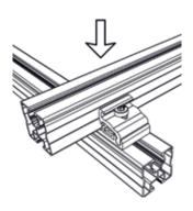
Mounting example with cross connector Rapid. Further information can be obtained in the respective mounting instruction (cross connector Rapid or cross connector KlickTop).
